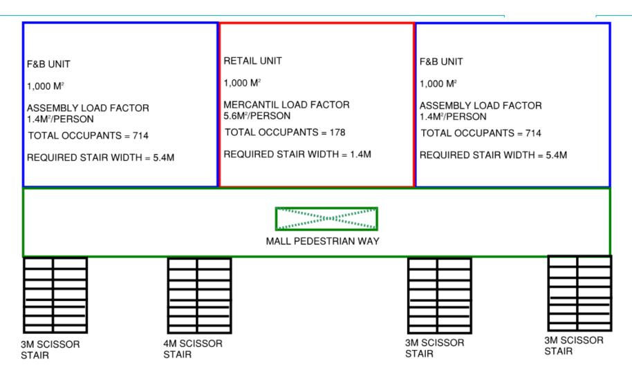
TOTAL REQUIRED STAIR WIDTH = 12.2M 12.2M = 4 SCISSOR STAIR 3M IN WIDTH EACH
