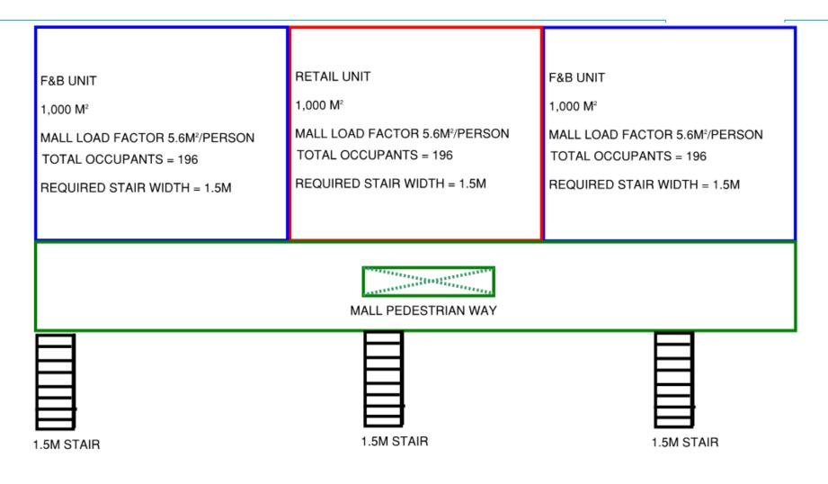
TOTAL REQUIRED STAIR WIDTH = 4.5M 4.5M = 3 STAIRS 1.5M IN WIDTH EACH
